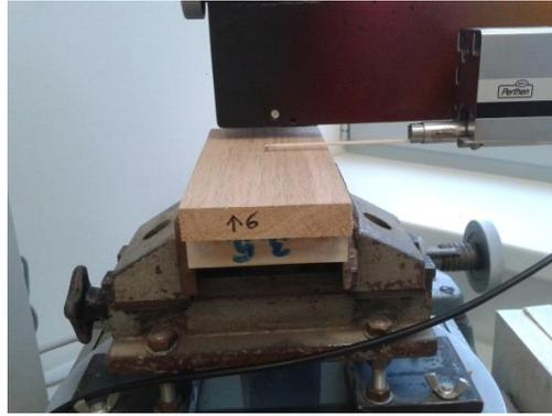
Figure 1. The S3P Perthometer with the stylus tip
