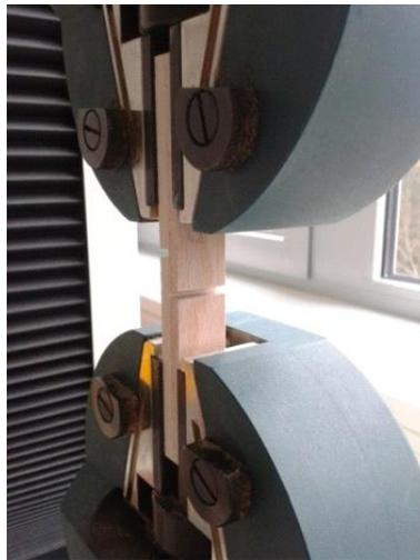
Figure 7. TiniusOlsen H10K instrument with a sample
